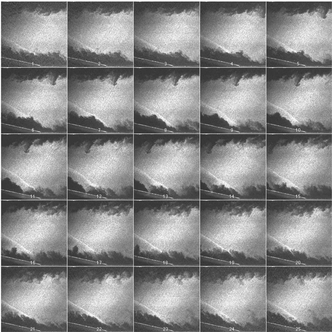
Fig. 11 Sequence of 25 streamwise view images of Mach 2.5 flow over 14-deg wedge. Flow is from right to left with 2\theta s between images.
